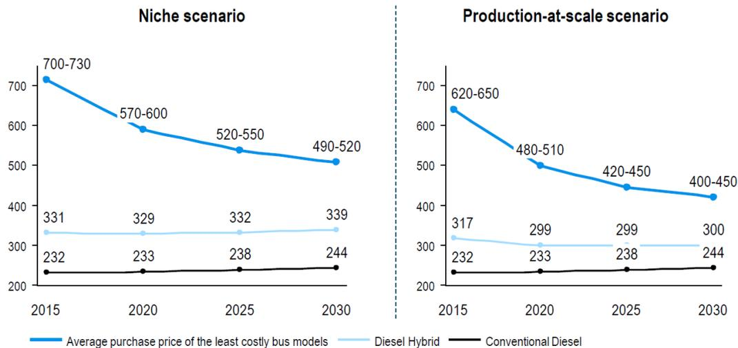
**Figure 3:** Fuel Cell bus cost. Niche scenario and production-at-scale scenario from fuel cell busses compared to Diesel and Diesel Hybrid busses. (Source: FCH-JU, Roland Berger, Fuel Cell Electric Buses). The expected costs for a fuel cell bus are currently 650.000 €.
