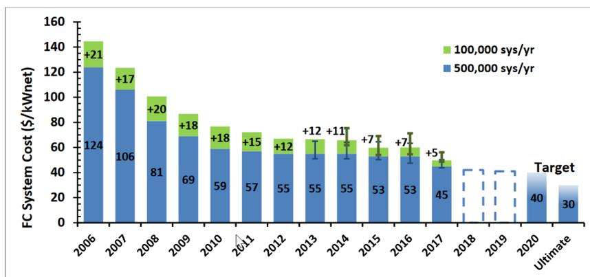
**Figure 4:** Modelled cost of an 80-kW<sub>net</sub> PEM fuel cell system based on projection to high-volume manufacturing (100,000 and 500,000 units/year). Source: Department of energy, Hydrogen and Fuel Cells Program Record 2018
