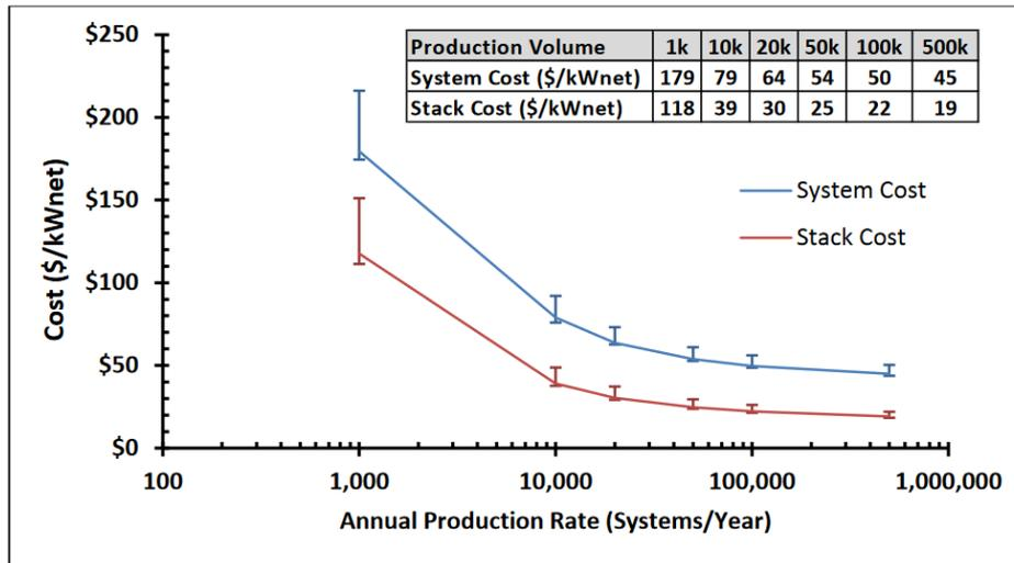
**Figure 5:** Projected cost of 2017 80-kW<sub>net</sub> transportation fuel cell stacks and systems at 1,000, 10,000, 20,000, 50,000, 100,000, and 500,000 units/year
