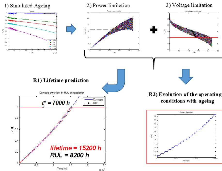
**Figure 2:** PEMFC RUL and operating conditions evaluation: 1) simulation; 2) power constraint coupled with 3) voltage limitation; R1) RUL extrapolation; R2) change in operating conditions.
